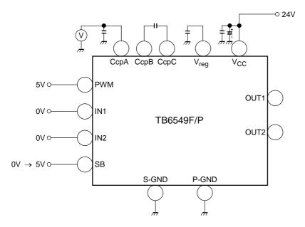
• tong: SB = 0 V  $\rightarrow$  5 V. Measure the time to boost CcpA voltage up about 29 V (24 V + 5 V)
