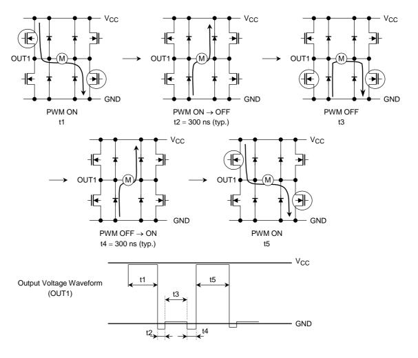
Note: Please set the pin PWM to High when PWM control function is not used.
