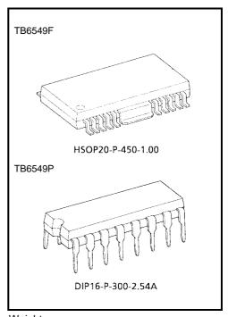
Weight HSOP20-P-450-1.00: 0.79 g (typ.) DIP16-P-300-2.54A: 1.11 g (typ.) DIP16-P-300-2.54A
