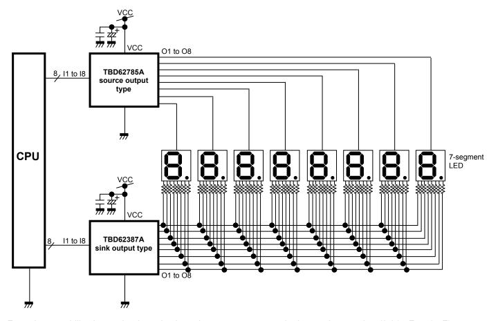
For voltage stabilization and noise rejection, please connect a stacked ceramic capacitor (0.01  $\mu$ F to 1  $\mu$ F) or an electrolytic capacitor (10  $\mu$ F to 100  $\mu$ F) to VCC line. The capacitor is recommended to be connected as close to the IC as possible.
