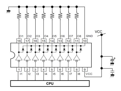
For voltage stabilization and noise rejection, please connect a stacked ceramic capacitor (0.01  $\mu$ F to 1  $\mu$ F) or an electrolytic capacitor (10  $\mu$ F to 100  $\mu$ F) to VCC line. The capacitor is recommended to be connected as close to the IC as possible.
