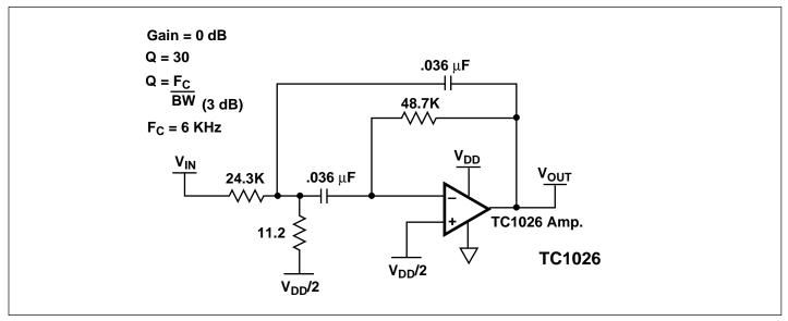
Figure 4. Second Order SAT Bandpass Filter
