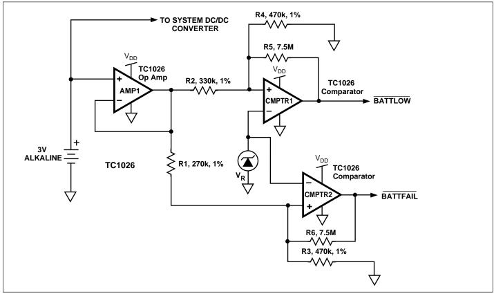
Figure 2. Precision Battery Monitor
