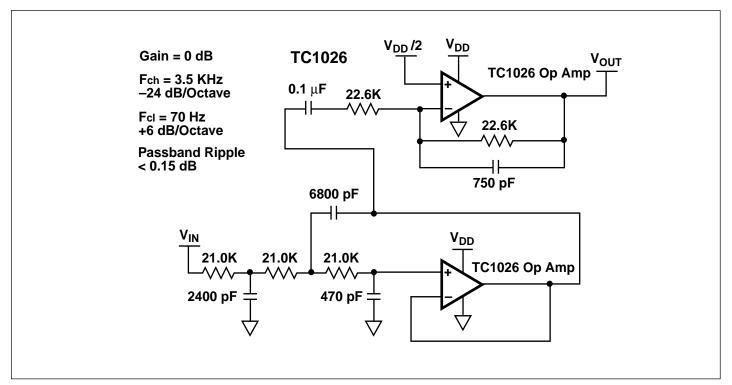
Figure 3. Multi-Pole Butterworth Voice Band Receive Filter
