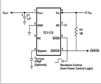
Figure 1: Typical Application Circuit
