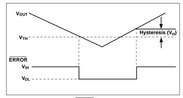
Figure 2: ERROR Output Operation
