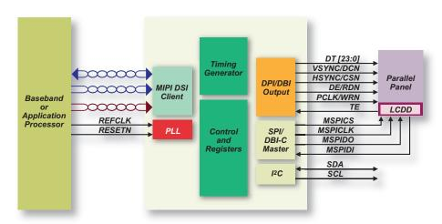
The TC358762XBG supports data transfer from input port to output port as shown in the following use case scenarios:
