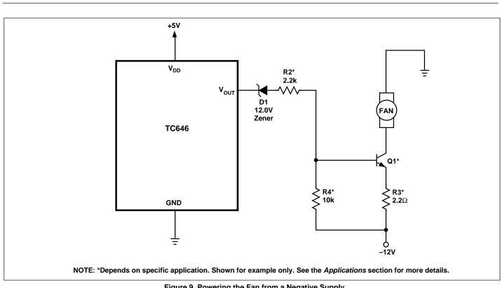
Figure 9. Powering the Fan from a Negative Supply
