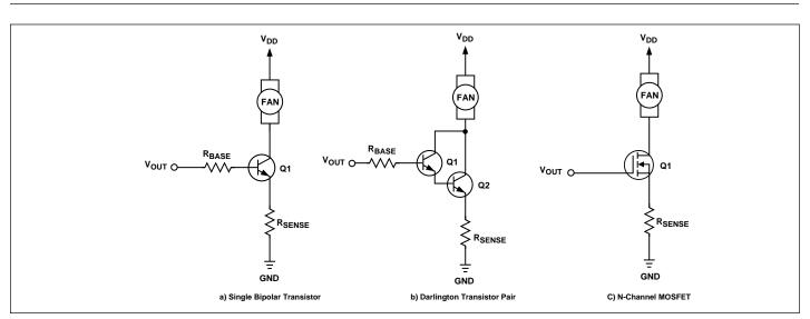
Figure 8. Output Drive Transistor Circuit Topologies
