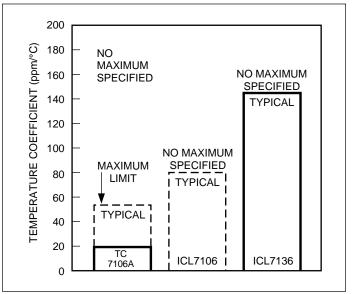
Figure 10. Analog Common Temperature Coefficient
