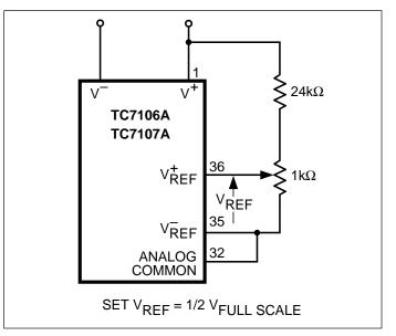
Figure 11. Internal Voltage Reference Connection
