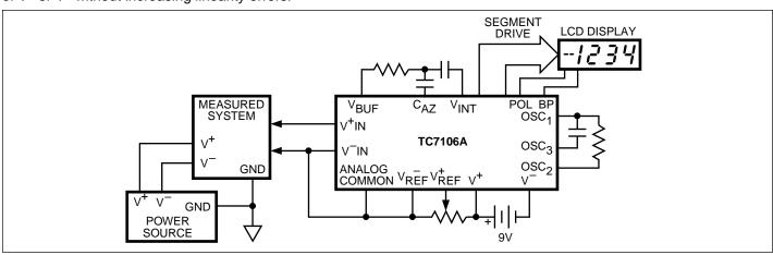
Figure 8. Common-Mode Voltage Removed in Battery Operation with Vin = Analog Common
