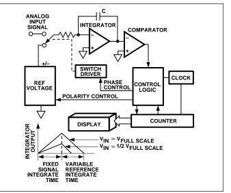
Figure 2A. Basic Dual Slope Converter
