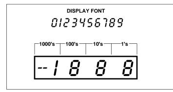
Figure 4. Display Font and Segment Assignment
