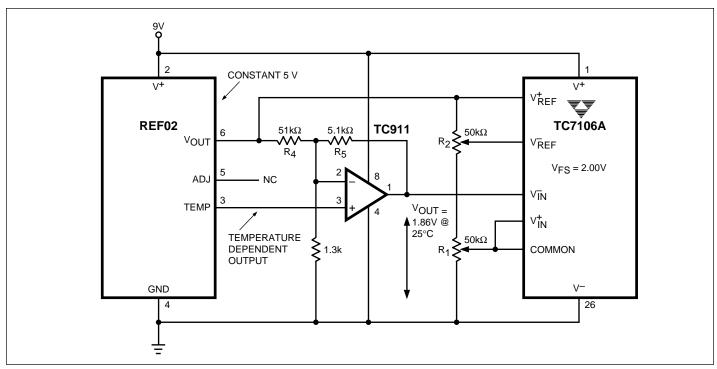
Figure 21. Integrated Circuit Temperature Sensor
