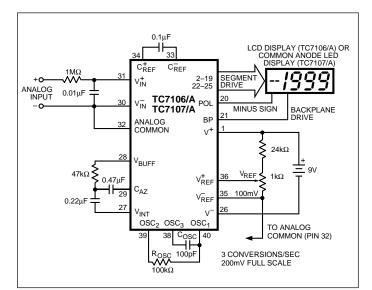
Figure 1. TC7106/A/7/A Typical Operating Circuit
