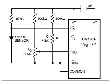
Figure 19. Temperature Sensor
