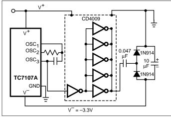
Figure 12. Generating Negative Supply From +5 V
