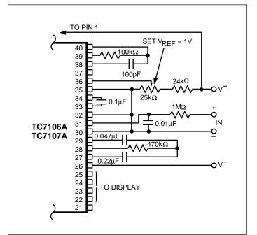
Figure 25. TC7106A/TC7107A: Recommended Component Values for 2.00V Full-Scale
