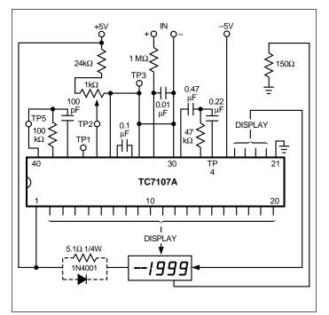
Figure 15. Diode or Resistor Limits Package Power Dissipation
