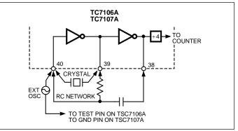
Figure 6. Clock Circuits
