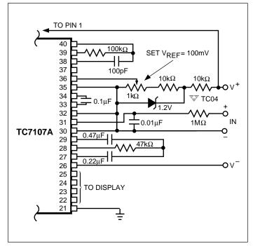
Figure 26. TC7107A With a 1.2V External Band-Gap Reference. ( $V_{\bar{I}N}$  Tied to Common.)
