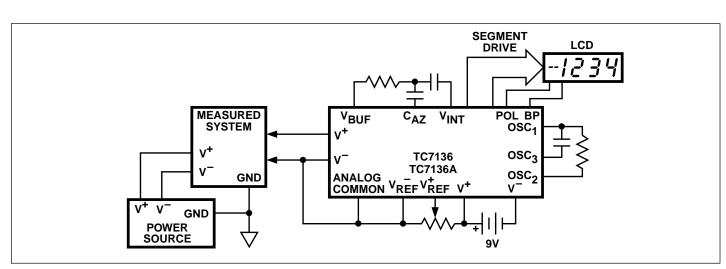
Figure 7. Common-Mode Voltage Removed in Battery Operation With VIN = Analog Common
