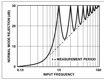
Figure 2. Normal-Mode Rejection of Dual-Slope Converter
