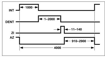
Figure 4. Conversion Timing During Normal Operation
