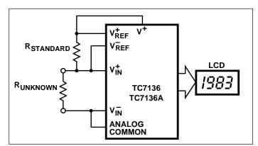
Figure 12. Low Parts Count Ratiometric Resistance Measurement
