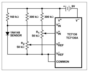
Figure 13. Temperature Sensor
