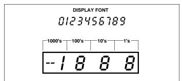
Figure 6. Display FONT and Segment Assignment
