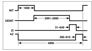
Figure 5. Conversion Timing During Overrange Operation
