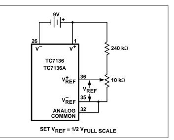
Figure 10. TC7136A Internal Voltage Reference Connection
