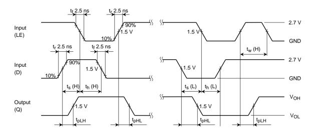
$\label{eq:Figure 2} \quad t_{pLH}, t_{pHL}, t_w, t_s, t_h$
