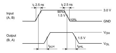
Figure 2 t<sub>pLH</sub>, t<sub>pHL</sub>
