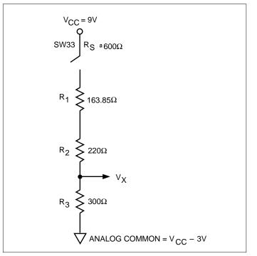
Figure 16. R $\Omega$ BUF Calculation (200  $\Omega$  Manual Operation)
