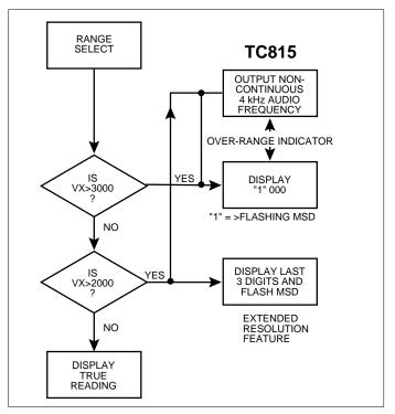
Figure 8. Manual Range Selection; Voltage Measurements
