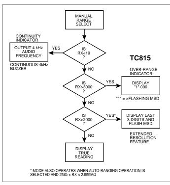
Figure 6. Manual Range Selection; Resistance Measurements
