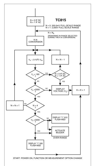
Figure 9. Auto-Range Operation; Voltage Measurement
