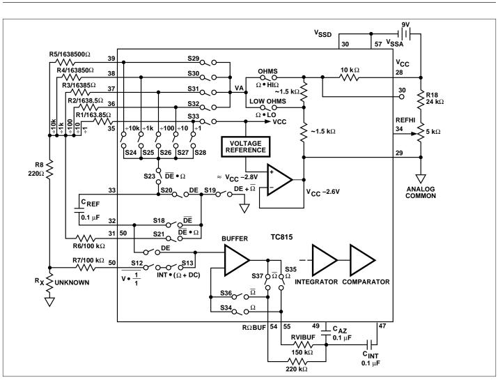
Figure 3: Ratiometric Resistance Measurement Functional Diagram
