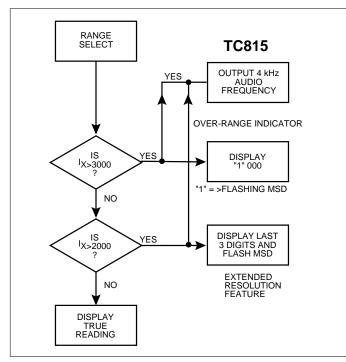
Figure 7. Manual Range Selection; Current Measurements
