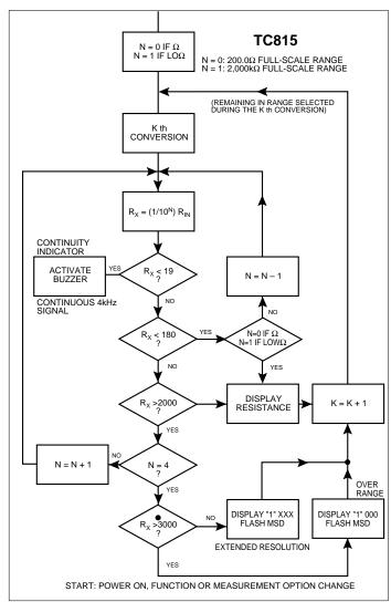
Figure 10. Auto-Range Operation; Resistance Measurement
