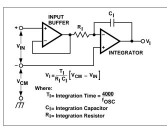
Figure 9. Common-Mode Voltage Reduces Available Integrator Swing (V<sub>COM</sub>  $\neq$  V<sub>IN</sub>)
