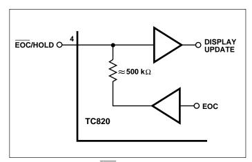
Figure 10. EOC/HOLD Pin Schematic
