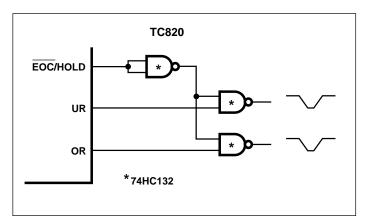
Figure 11. Generating Underrange and Overrange Pulses
