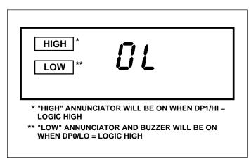
Figure 7. LCD During Logic Probe Operation
