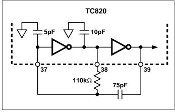
Figure 16. R-C Oscillator Circuit
