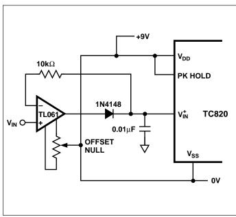
Figure 23. External Peak Detector
