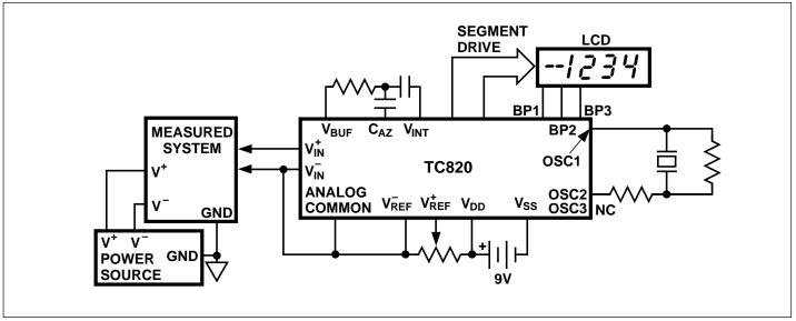
Figure 8. Common-Mode Voltage Removed in Battery Operation With  $V_{\overline{IN}}$  = Analog Common
