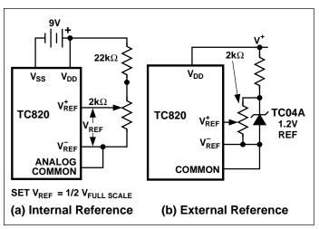
Figure 18. Reference Voltage Connections
