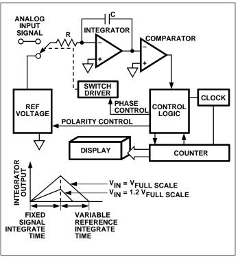
Figure 2. Basic Dual-Slope Converter
