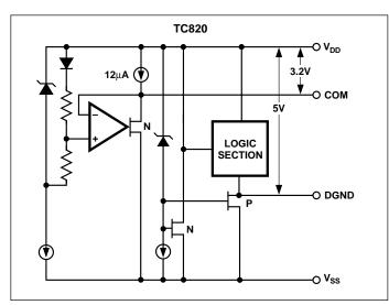
Figure 14. DGND and COM Outputs
