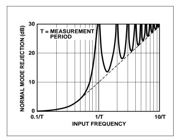
Figure 3. Normal-Mode Rejection of Dual-Slope Converter
