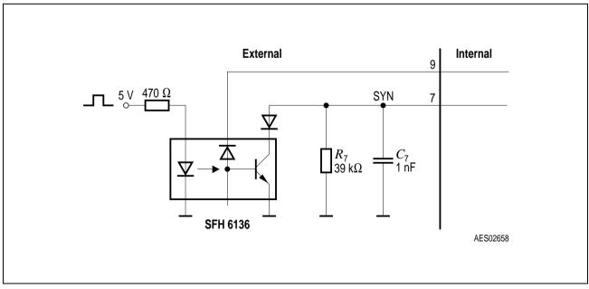
Figure 13 Ext. Synchronization Circuit
