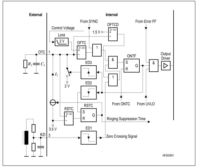
Figure 6 Off-Time-Circuit
