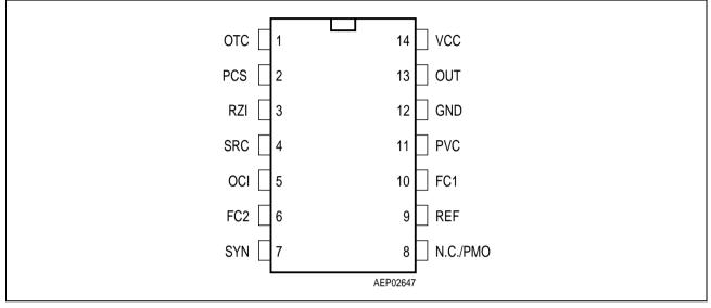
Figure 1 Pin Configuration (top view)
