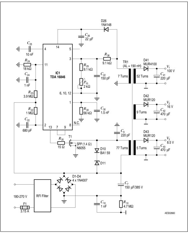
Figure 16 Circuit Diagram for Standard Application
