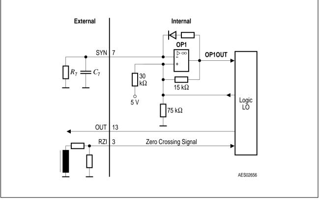
Figure 11 Synchronization and Fixed Frequency Circuit
