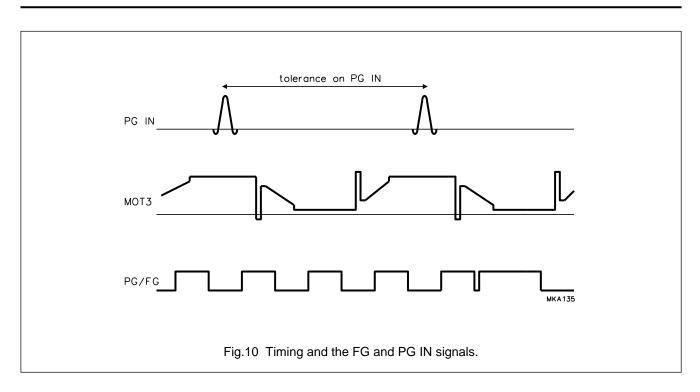
The special PG pulse is derived from the negative-going zero-crossing from the MOT3 output (pin 16). The external PG signal (PG IN on pin 5) must sense a positive-going voltage (>80 mV) within 1.5 to 7.5 commutation periods before the negative-going zero-crossing in MOT3 (see Fig.10).
