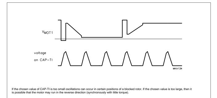
Fig.8 Typical CAP-TI and  $V_{\text{MOT1}}$  voltage waveforms in normal running mode.
