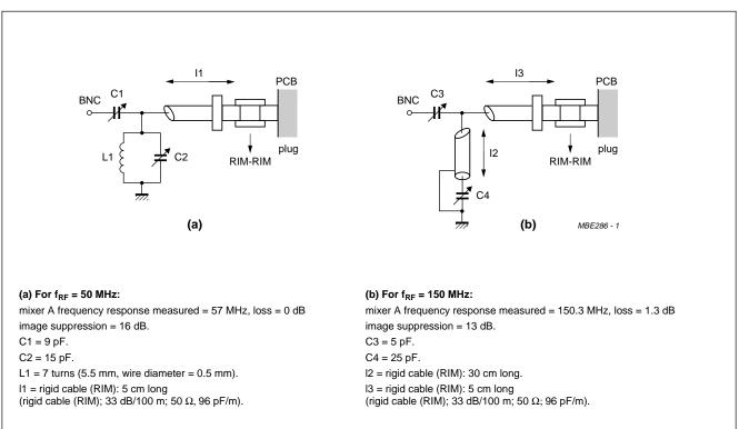
Fig.5 Input circuit for minimum noise figure.
