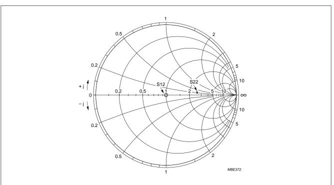
Fig.11 Reverse transmission and output reflection coefficient ( $S_{12}$  and  $S_{22}$ ) of the IF amplifier (25 to 45 MHz) (Z chart).
