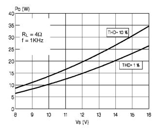
Figure 5: EIAJ power vs Supply Voltage
