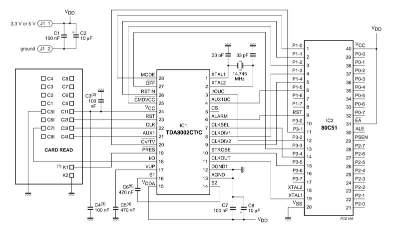
TDA8002C should be placed as close as possible to the card reader.
