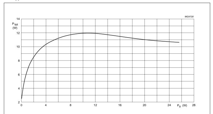
Fig.23 Total power dissipation as a function of output power;  $V_P$  = 14.4 V,  $R_L$  = 4  $\Omega$  (1 channel driven BTL or 4 channels in single-ended mode).
