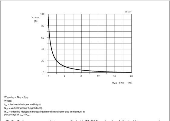
Fig.7 Static error on average histogram amplitude (pin TAUHM) as a function of effective histogram measuring time in a field.
