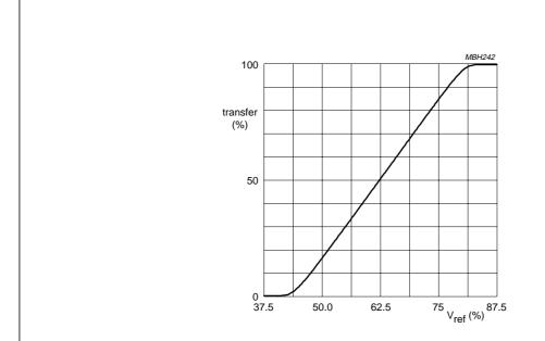
Fig.15 Feature setting control as a function of the pin voltage for peaking, coring, steepness and line width.
