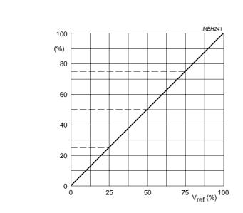
Fig.14 Relative increase of coring level as a function of voltage at pin SNC starting from four different coring level presets.
