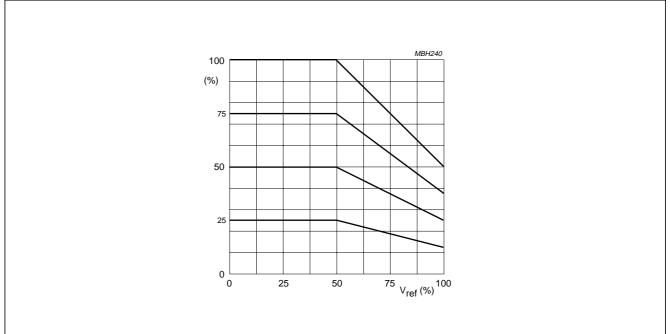
Fig.13 Relative decrease of steepness level as a function of voltage at pin SNC starting from four different
