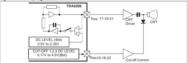
Figure 5. DC Coupling with Cut-off Control
