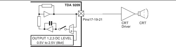
Figure 7. DC Coupling with Feedback (LCD mode)
