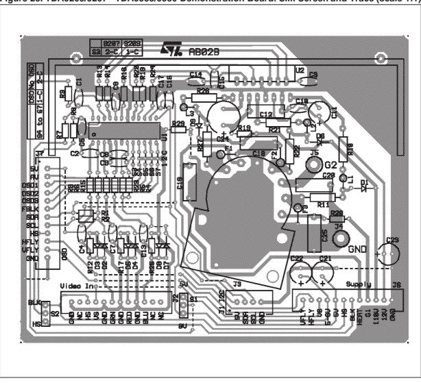
Figure 23. TDA9209/9207 - TDA9533/9530 Demonstration Board: Silk Screen and Trace (scale 1:1)
