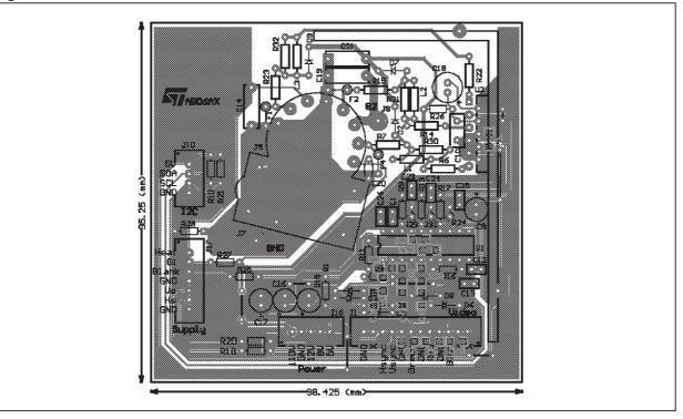
Figure 18. TDA9210 - TDA9535/9536 Demonstration Board: Silk Screen and Trace
