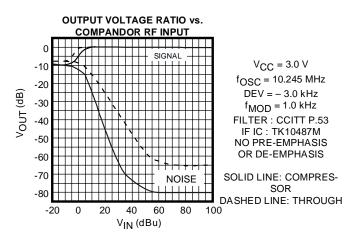
Finally, the overall characteristics are measured using both the compressor and the expander. The output is measured when the compressor's input is at  $-40 \text{ dB}\mu\text{V}$  and the frequency deviation is  $\pm 3.0 \text{ kHz}$ .
