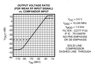
The following graph shows the characteristics when the RF input is weak (RF IN =  $30 \text{ dB}\mu$ ). There is a great difference when the compandor is used with a weak RF input. When the through function is used (noise reduction off), the output is lost in noise as the compressor input drops below -80 dBV; but when the compandor function is used, it remains level below -100 dBV. With a weak RF input, dynamic range is extended by 30 dB.
