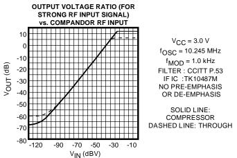
The effects of the compandor within a narrow band FM communications system was demonstrated while a coaxial cable was used in place of transmission through free space. The signal source was an FM signal generator although there are some differences when actual transmission is through free space. However, the test configuration used in this experiment is useful in understanding the effects of the compandor.
