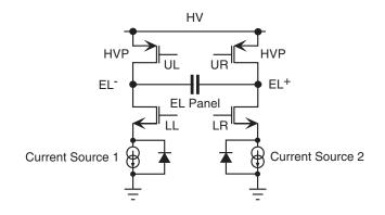
FIGURE 2: H-BRIDGE SCHEMATIC
