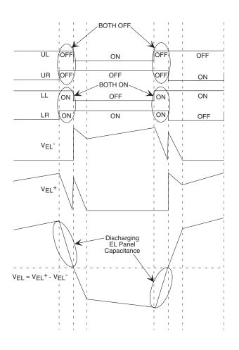
FIGURE 3: H-BRIDGE SEQUENCING WAVEFORMS
