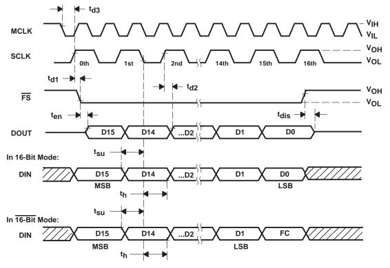
Figure 3–1. Primary Serial Communication Timing
