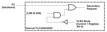
Figure 3–3. Hardware and Software Methods to Initate a Secondary Request
