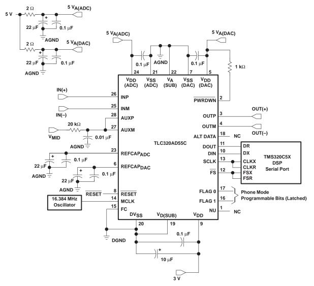
Figure 5–2. TLC320AD55C I/O Buffer and V<sub>MID</sub> Generator Schematic
