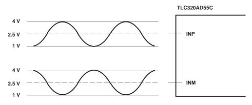
Figure 2–3. Differential Analog Input Configuration
