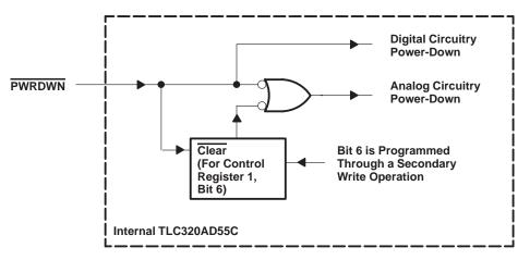
Figure 2–2. Internal Power-Down Logic
