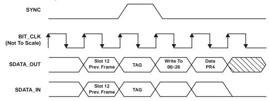
Figure 2-4. TLC320AD90C Power-Down Mode Timing
