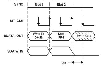
Figure 4–1. AC-Link Low-Power Mode Timing
