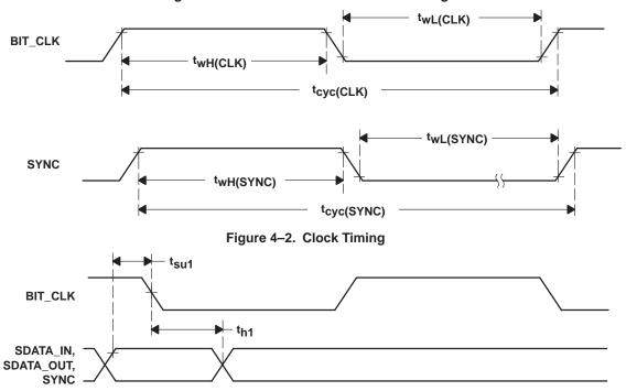
Figure 4-3. Data Setup and Hold Timing
