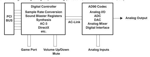
Figure 5-1. System Diagram
