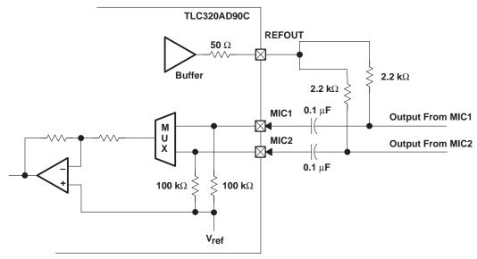
Figure 2-7. Microphone Programmable Gain Amplifier With Two Electret Microphones
