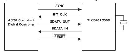
Figure 5-2. Connection to an AC'97 Digital Controller
