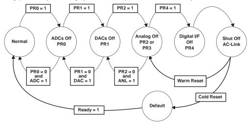
Figure 2-8. TLC320AD90C Power-Down/ Power-Up Flow Example
