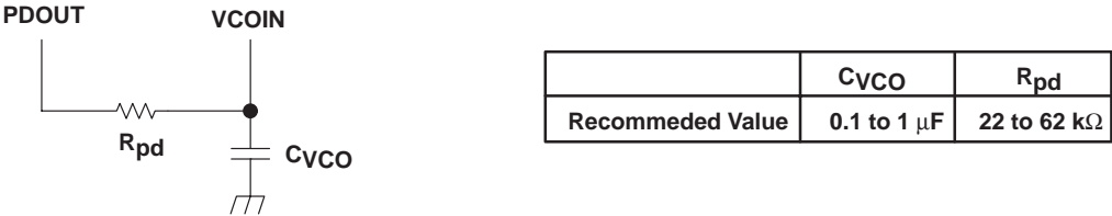
Figure 8. Resistor and Capacitor Connection
