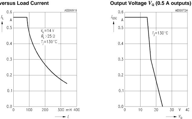
When switching the maximum inductive loads, the maximum temperature  $T_j$  of 150 °C may be briefly exceeded. The IC will not be destroyed by this, but the restrictions concerning useful life should be observed.
