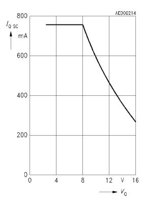
Maximum permissible output currents, being the result of the typical thermal power dissipation in a **P-DIP-8-1** package, for three operating modes.
