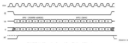
FIGURE 13. Microwire Control Port Timing: MW = 1
