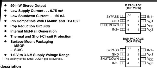
The TPA6100A2 is a stereo audio power amplifier packaged in either an 8-pin SOIC package or an 8-pin MSOP package capable of delivering 50 mW of continuous RMS power per channel into  $16-\Omega$  loads. Amplifier gain is externally configured by a means of three resistors per input channel and does not require external compensation for settings of 1 to 10.
