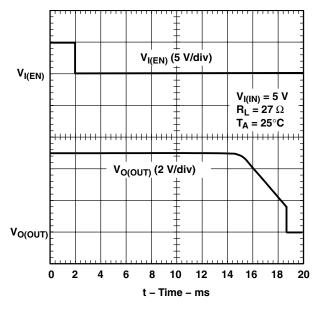
Figure 3. Turnoff Delay and Fall Time
