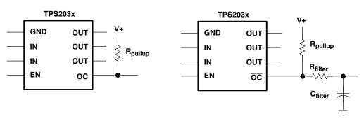
Figure 39. Typical Circuit for OC Pin and RC Filter for Damping Inrush OC Responses
