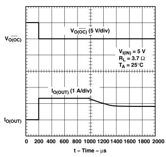
Figure 15. 3.7- $\Omega$  Load Connected to an Enabled TPS2031 Device
