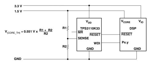
Figure 13. TPS3110 in a DSP System Monitoring Both Supply Voltages
