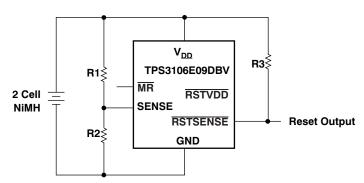
Figure 11. Battery Monitoring with 3-μA Supply Current for Device and Resistor Divider
