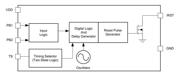
Figure 2. Block Diagram
