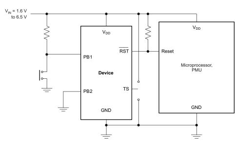
NOTE: Connect TS to V<sub>DD</sub> or ground for different PB time delays. Connect one PB input to ground for use as a single channel.
