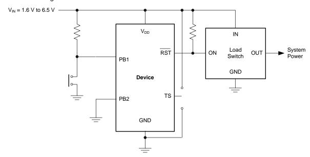
NOTE: Connect TS to V<sub>DD</sub> or ground for different PB time delays. Connect one PB input to ground for use as a single channel.
