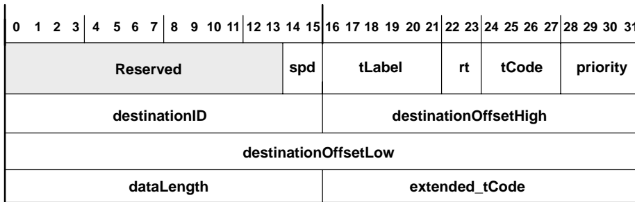
Figure 4–6. Block-Transmit Format (Read Request)
