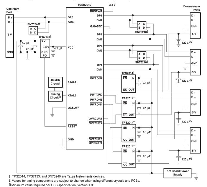
Figure 10. TUSB2040 Self-Powered Hub, Individual-Port Power Management Application
