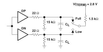
Figure 1. Differential Driver Switching Load
