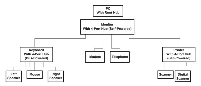
Figure 7. USB Tiered Configuration Example
