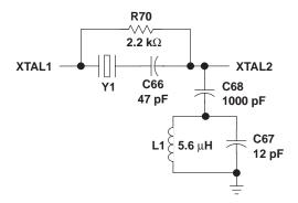
NOTES: C. When tuning the crystal (Y1) for different board implementations, the capacitor (C67) is subject to change. Other components should remain the same. **Figure 6. Tuning Circuit**
