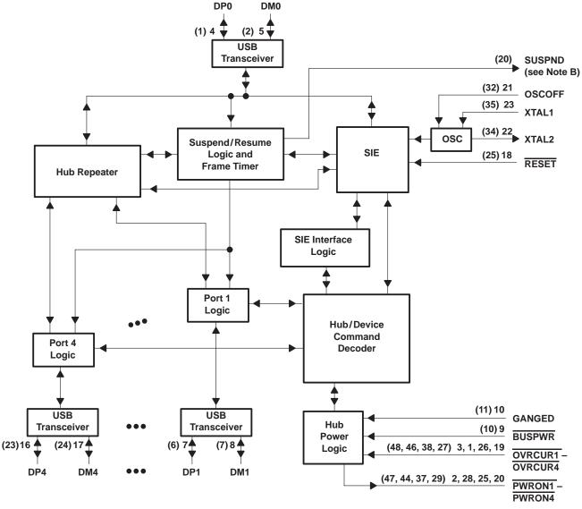
NOTES: A. Pins in parentheses are for TQFP package
