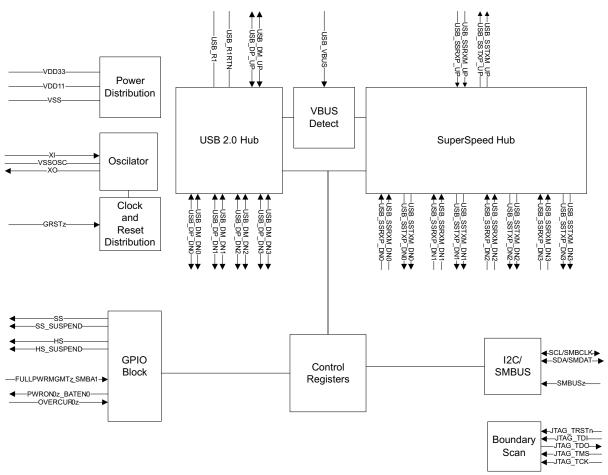
Figure 1-2. TUSB8040PFP Functional Block Diagram
