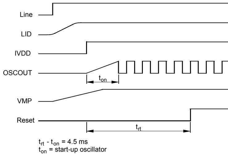
**Figure 10.** Power-on Reset (Ringing)
