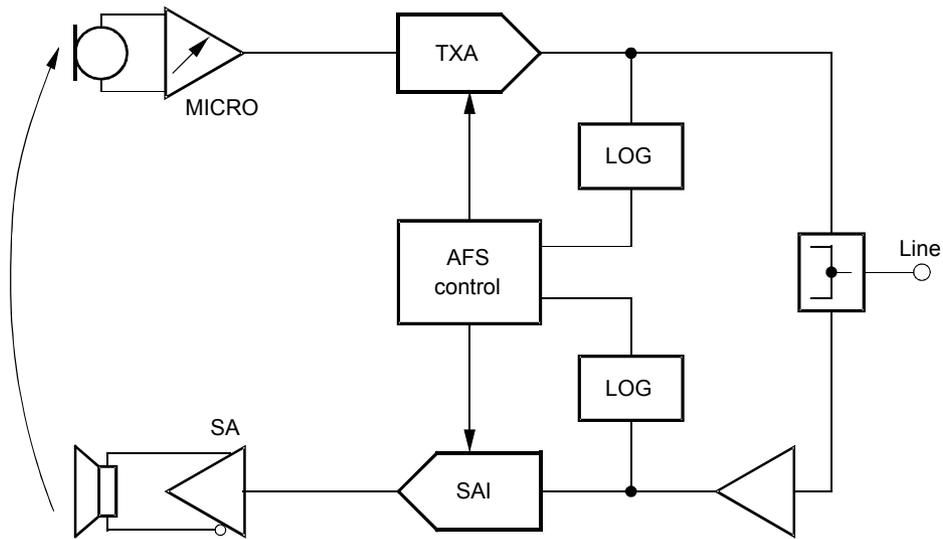
**Figure 16.** Block Diagram Hands-free Mode U4091BM-N 4-point Signal Sensing
