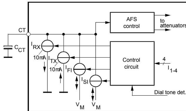
**Figure 15.** Block Diagram Hands-free Mode U4091BM-N 2-point Signal Sensing
