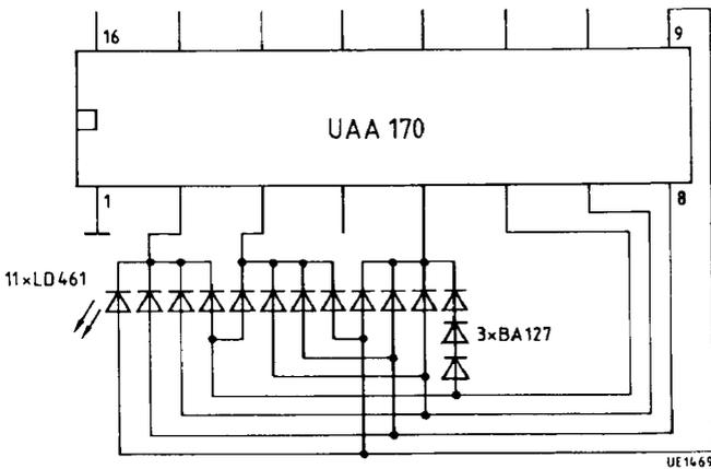
**Application Circuit for the Control of 30 LEDs with 2 × UAA 170**
