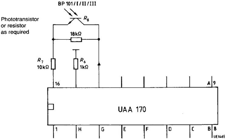
Pins 14, 15, and 16 serve to determine the diode current. Corresponding to the desired light intensity, the forward current of the diodes is linearly variable in the range  $I_D$  approx. 0 to 50 mA. The resistance at pin 15 defines the adjusting range. The resistances between pin 14 and 16 determine the current.
