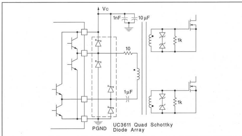
Figure 5. Transformer Coupled Push-Pull MOSFET Drive Circuit
