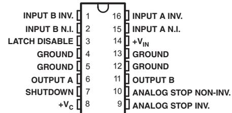
NOTE: All four ground pins must be connected to a common ground.
