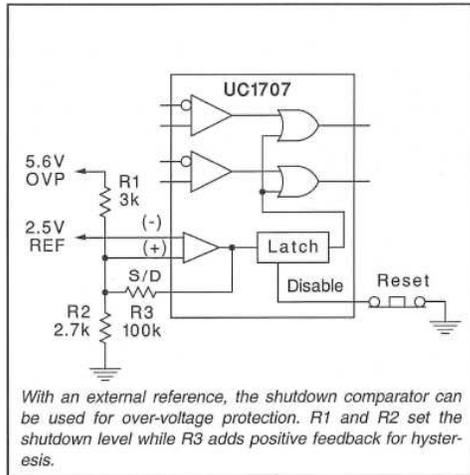
Figure 7. Over-Voltage Protection
