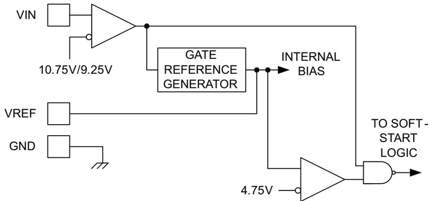
Figure 3. Undervoltage Circuit
