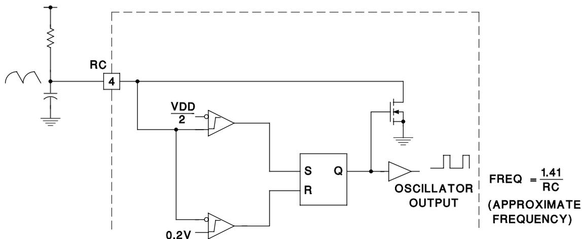
NOTE: The oscillator generates a sawtooth waveform on RC. During the RC rise time, the output stages alternate on time, but both stages are off during the RC fall time. The output stages switch a 1/2 the oscillator frequency, with guaranteed duty cycle of < 50% for both outputs.
