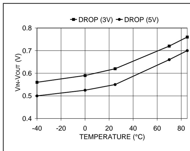
Figure 4. Typical dropout vs. temperature (1A load).
