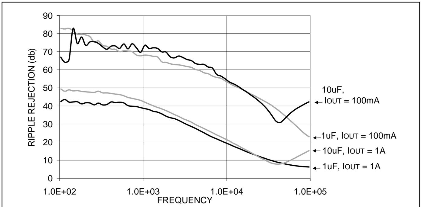
Figure 5. Ripple rejection vs. frequency.
