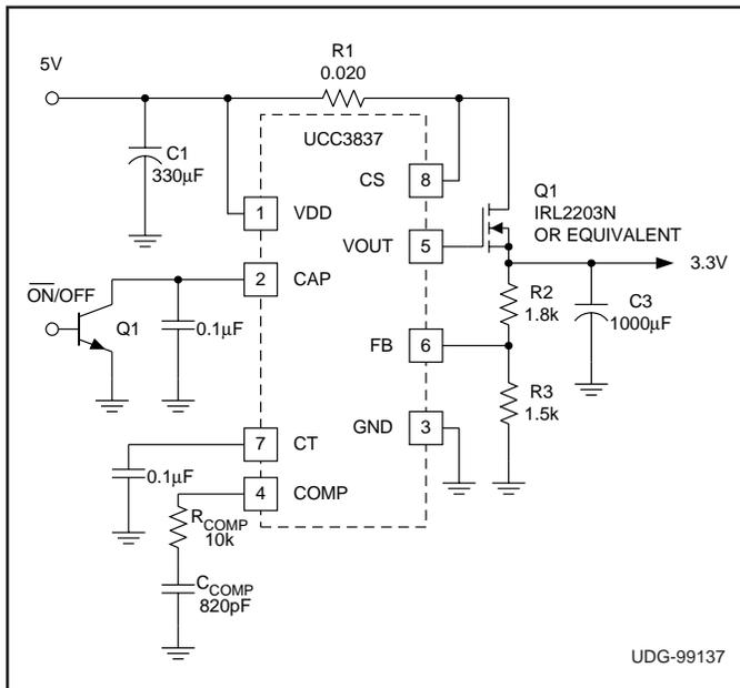
Figure 1. Typical application 5V to 3.3V, 5A
