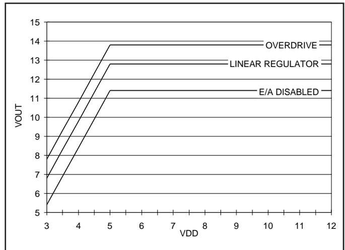
Figure 2. Typical V<sub>OUT(max)</sub> vs. VDD.
