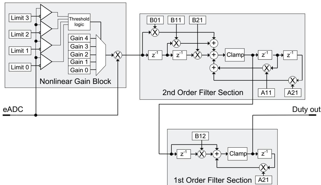
**Figure 9. Digital Compensator**
