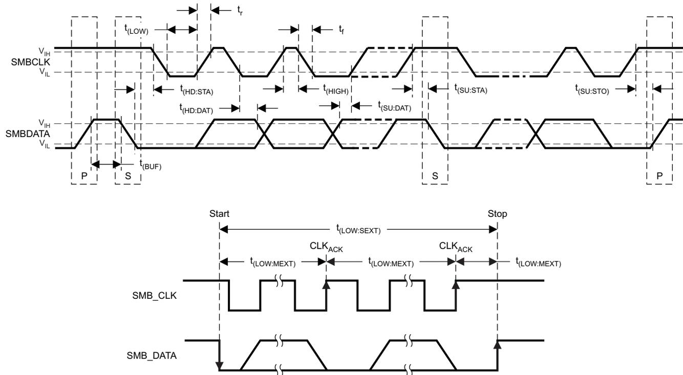
Figure 1. I<sup>2</sup>C/SMBus/PMBus Timing in Extended Mode Diagram
