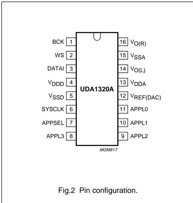
Fig.2 Pin configuration.
