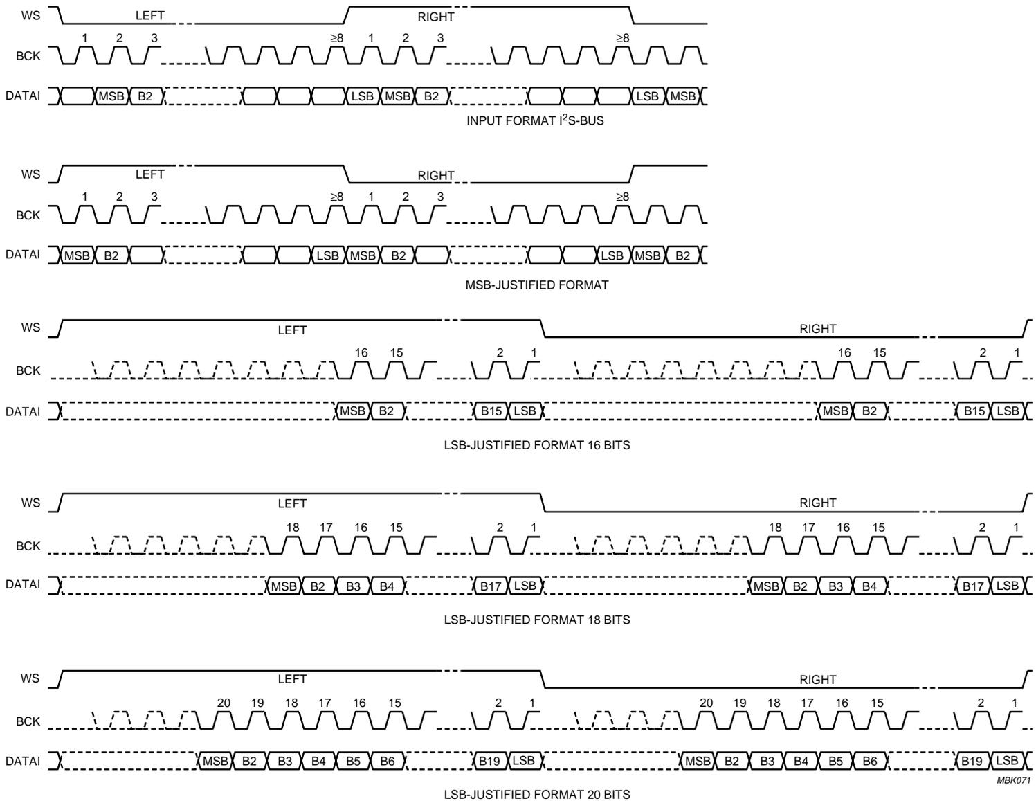
Fig.3 Serial interface; input format I<sup>2</sup>S-bus.
