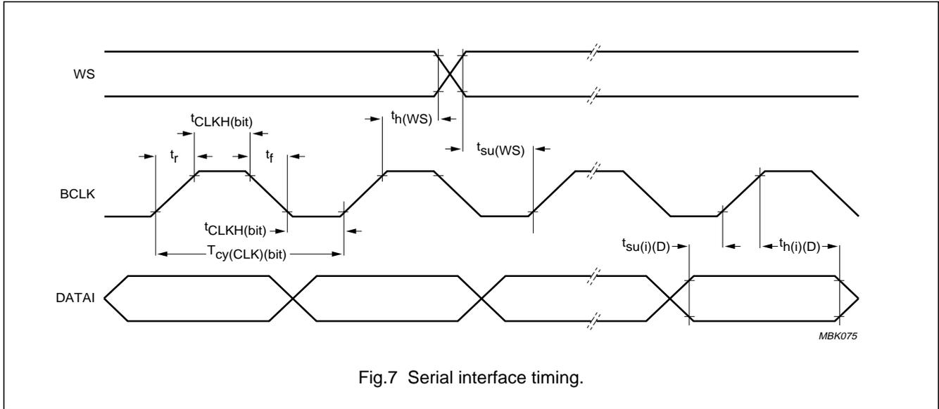
Fig.7 Serial interface timing.
