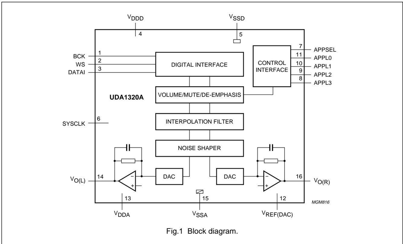
Fig.1 Block diagram.
