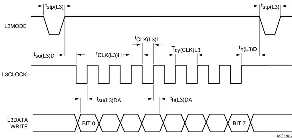
Fig.11 Timing for data transfer mode.
