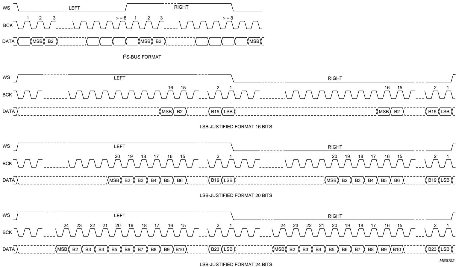
Fig.6 Digital data interface formats.
