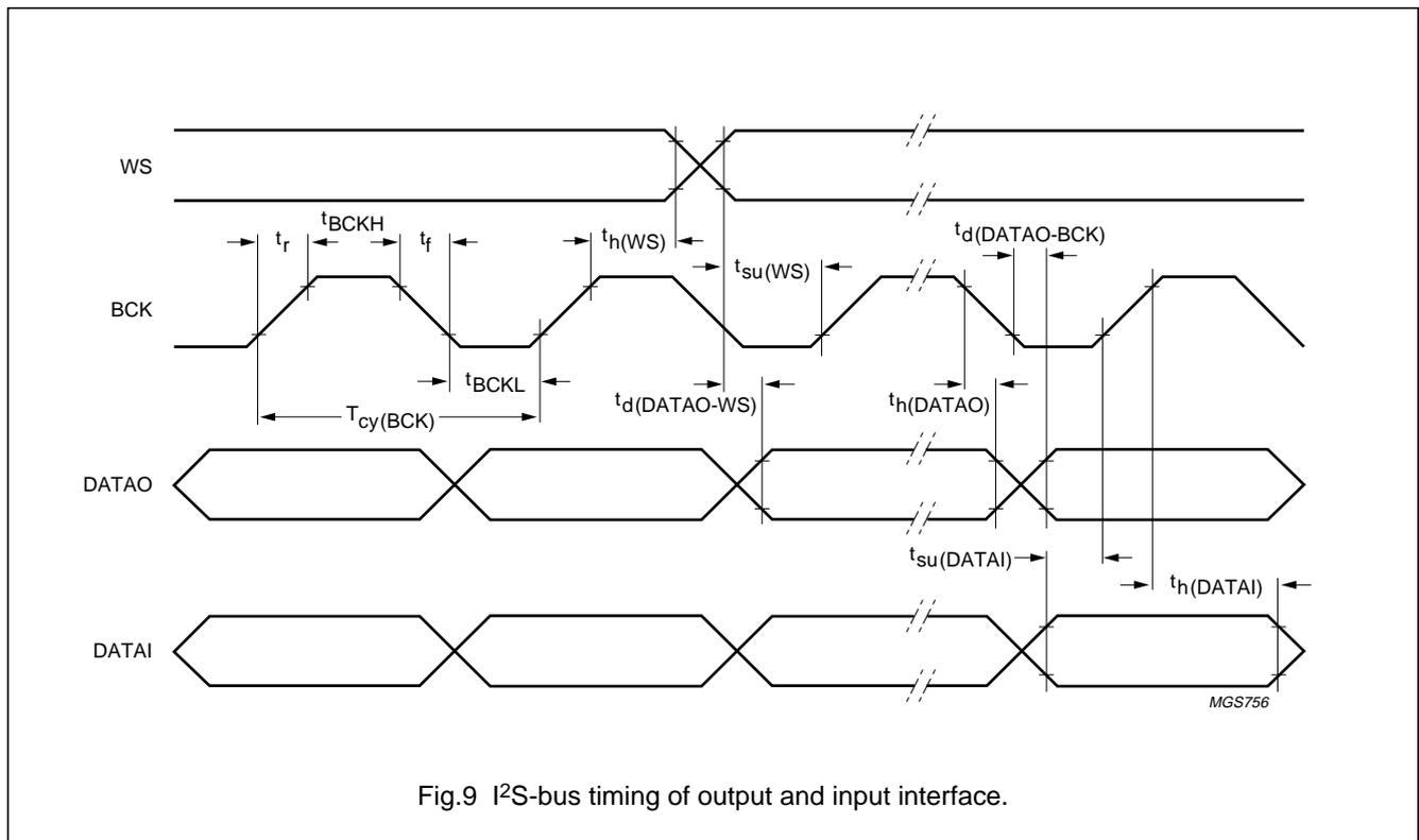
Fig.9 I<sup>2</sup>S-bus timing of output and input interface.
