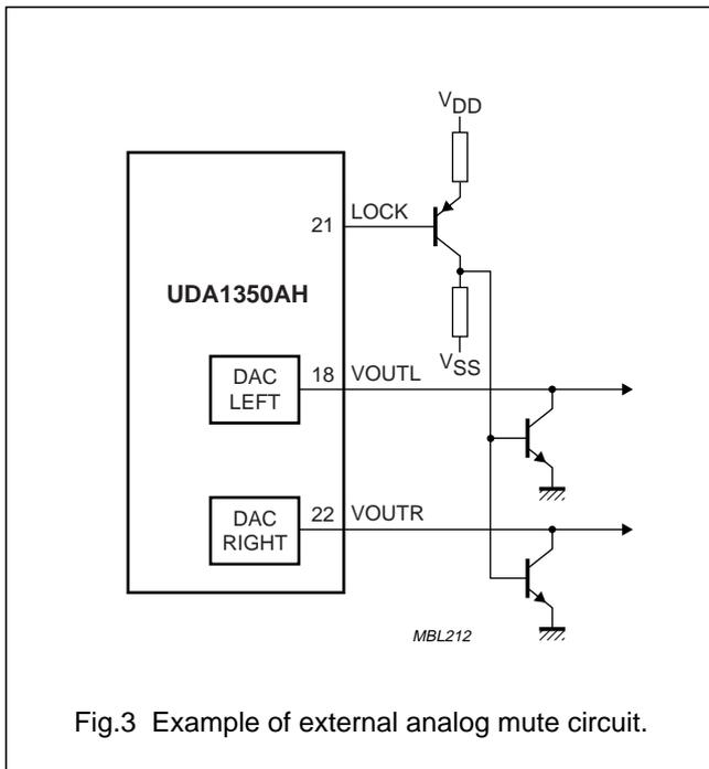
Fig.3 Example of external analog mute circuit.
