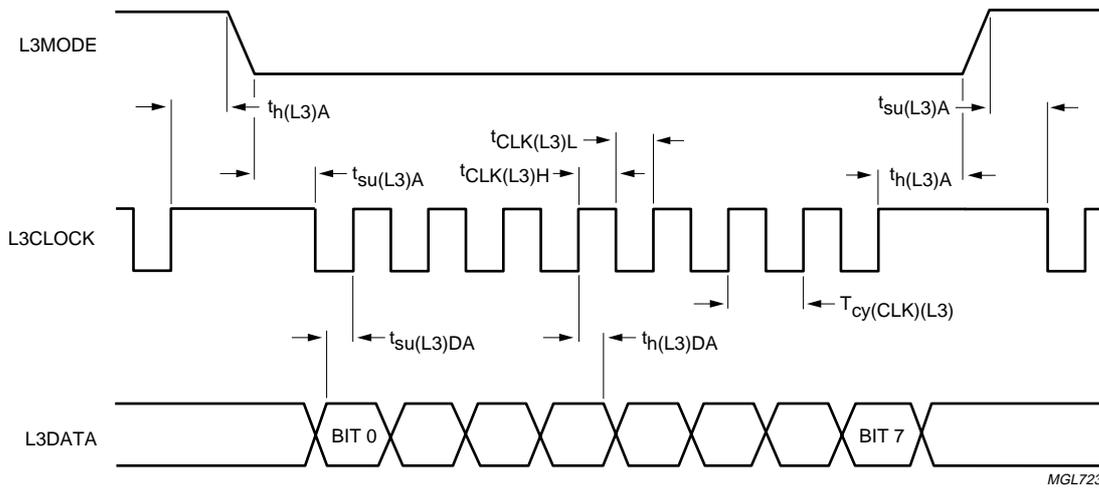
Fig.10 Timing for address mode.
