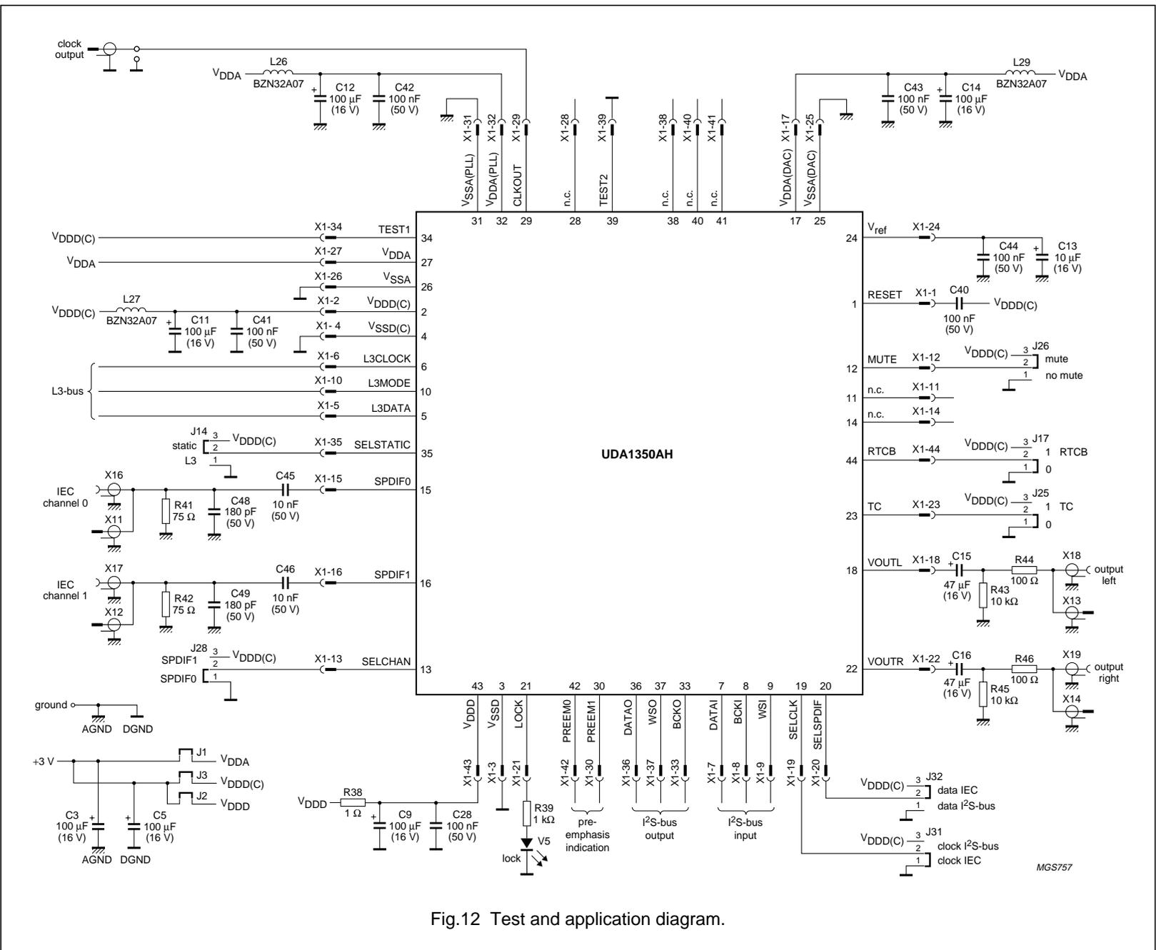
Fig.12 Test and application diagram.
