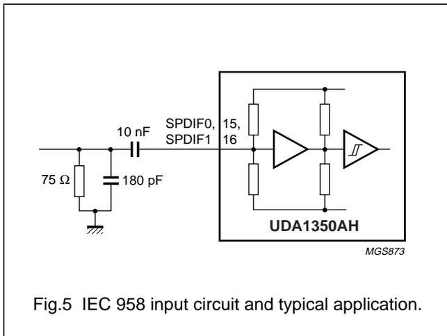
All 24 bits of data for left and right are extracted from the input bitstream as well as several of the IEC 958 key channel-status bits.
