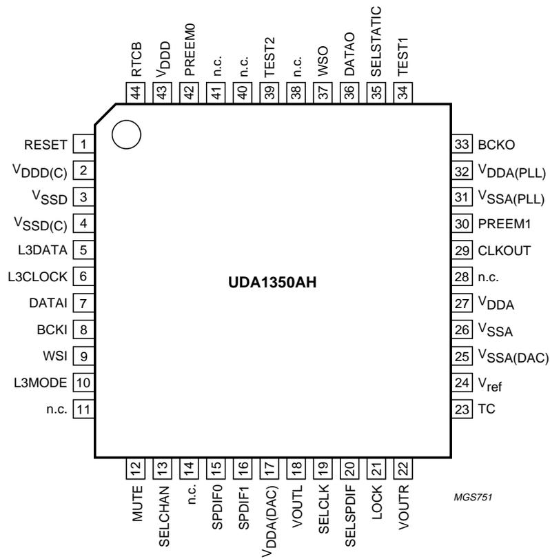
Fig.2 Pin configuration.
