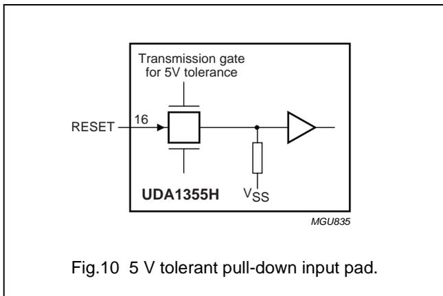
Fig.10 5 V tolerant pull-down input pad.
