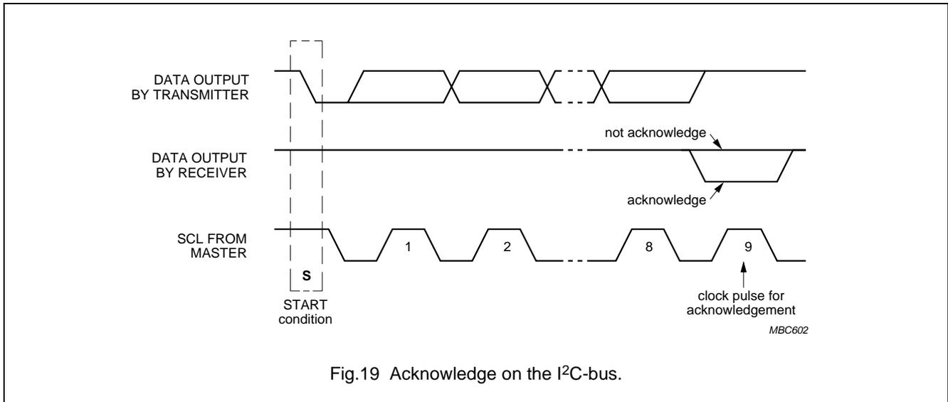
Fig.19 Acknowledge on the I<sup>2</sup>C-bus.
