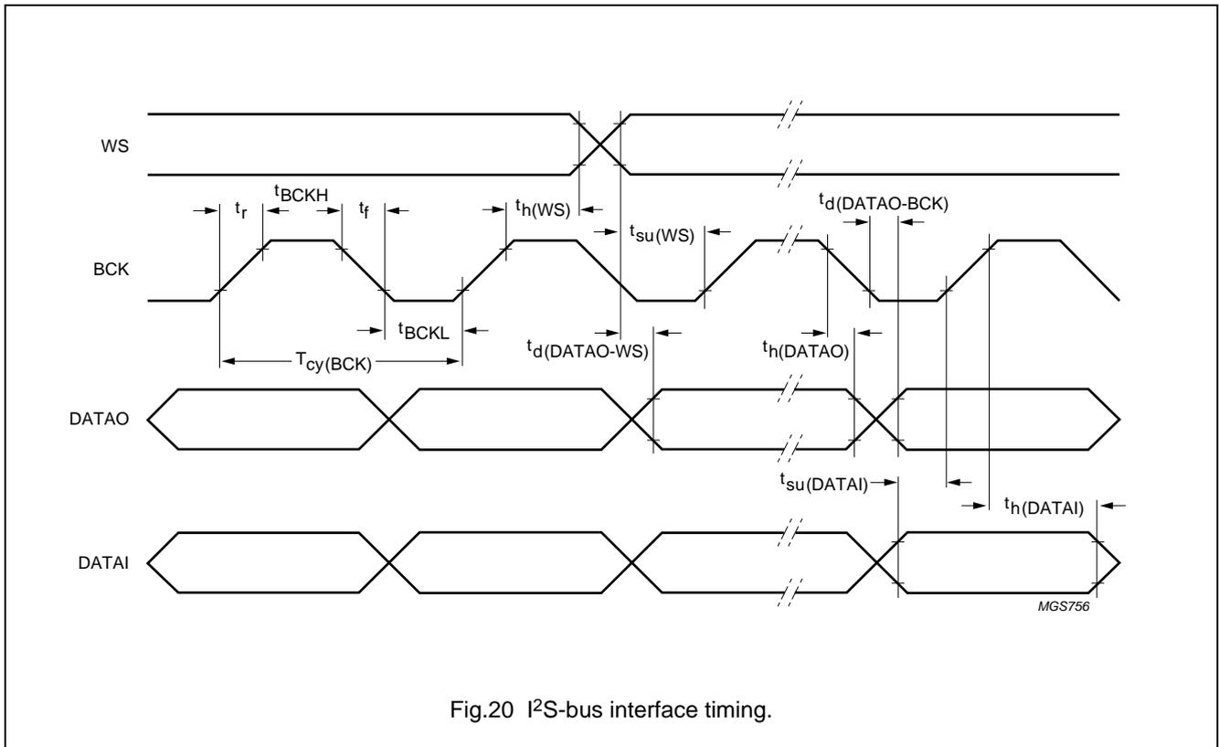
Fig.20 I²S-bus interface timing.
