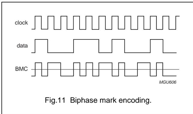
Fig.11 Biphasic mark encoding.
