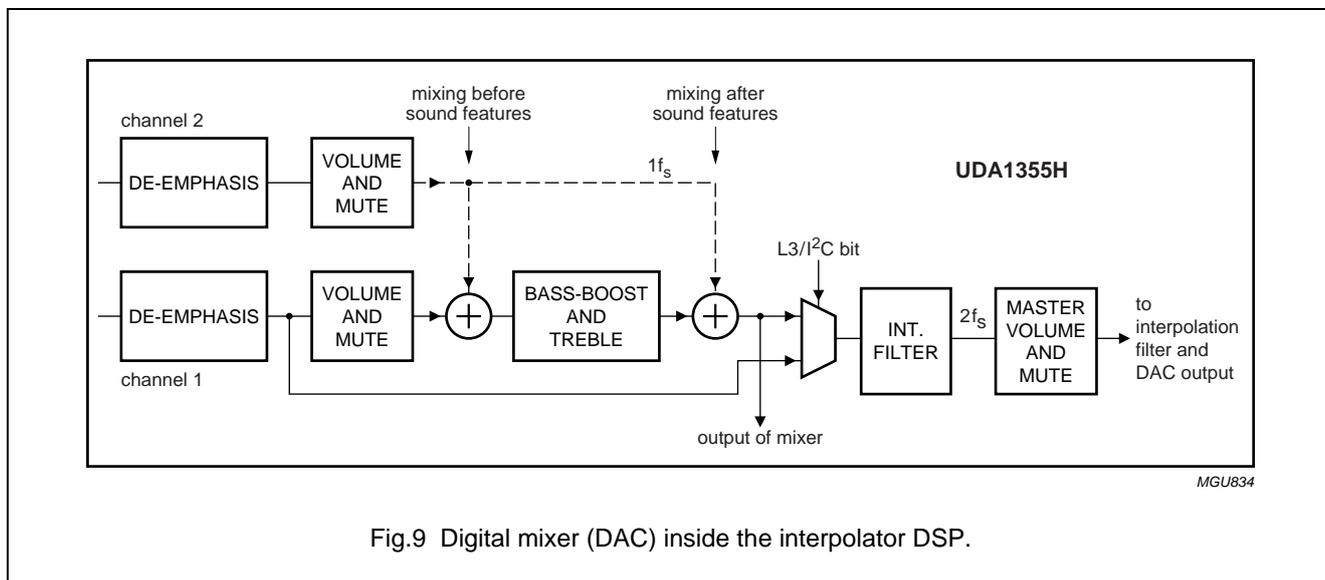
Fig.9 Digital mixer (DAC) inside the interpolator DSP.
