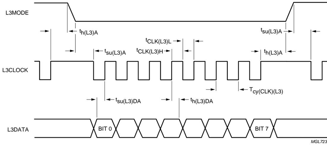
Fig.21 L3-bus interface timing for address mode.
