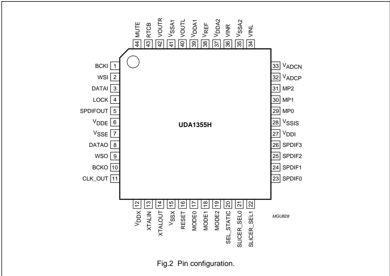
Fig.2 Pin configuration.
