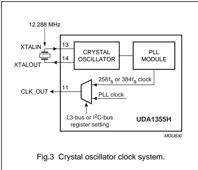
Fig.3 Crystal oscillator clock system.
