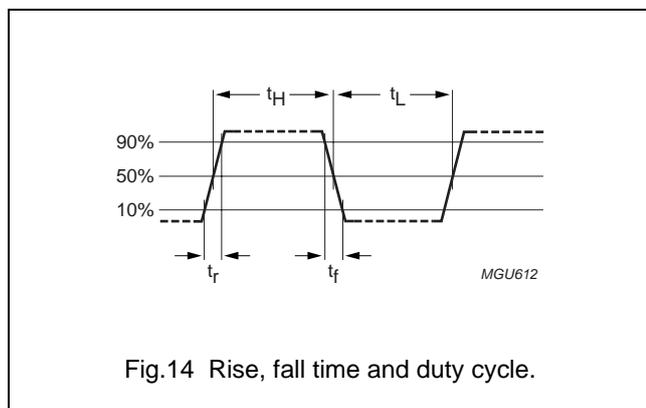
Fig.14 Rise, fall time and duty cycle.
