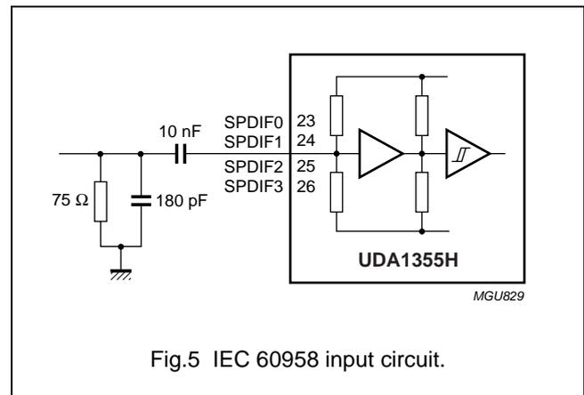
Fig.5 IEC 60958 input circuit.
