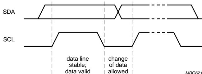
Fig.17 Bit transfer on the I<sup>2</sup>C-bus.
