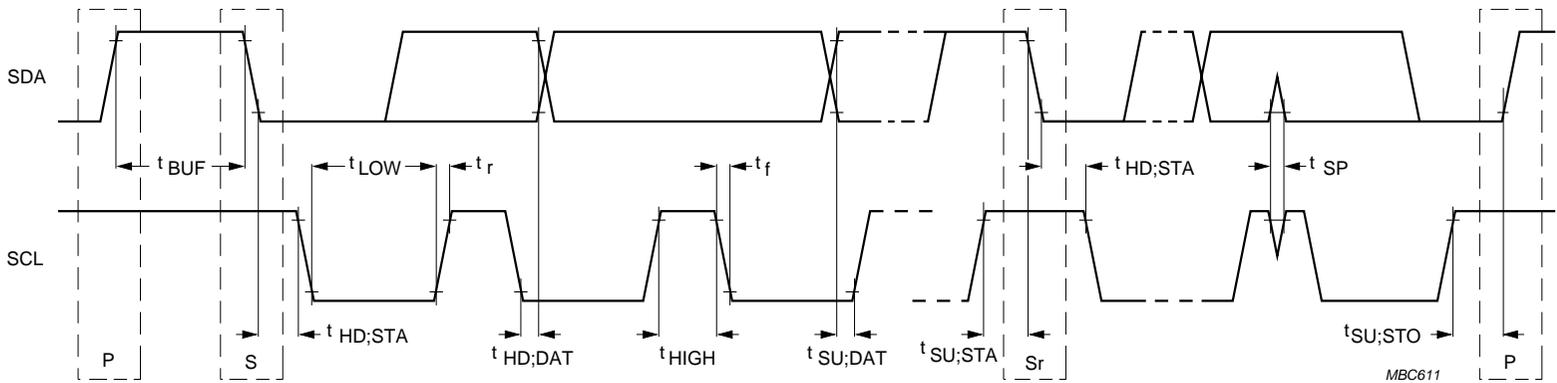
Fig.23 I<sup>2</sup>C-bus interface timing.
