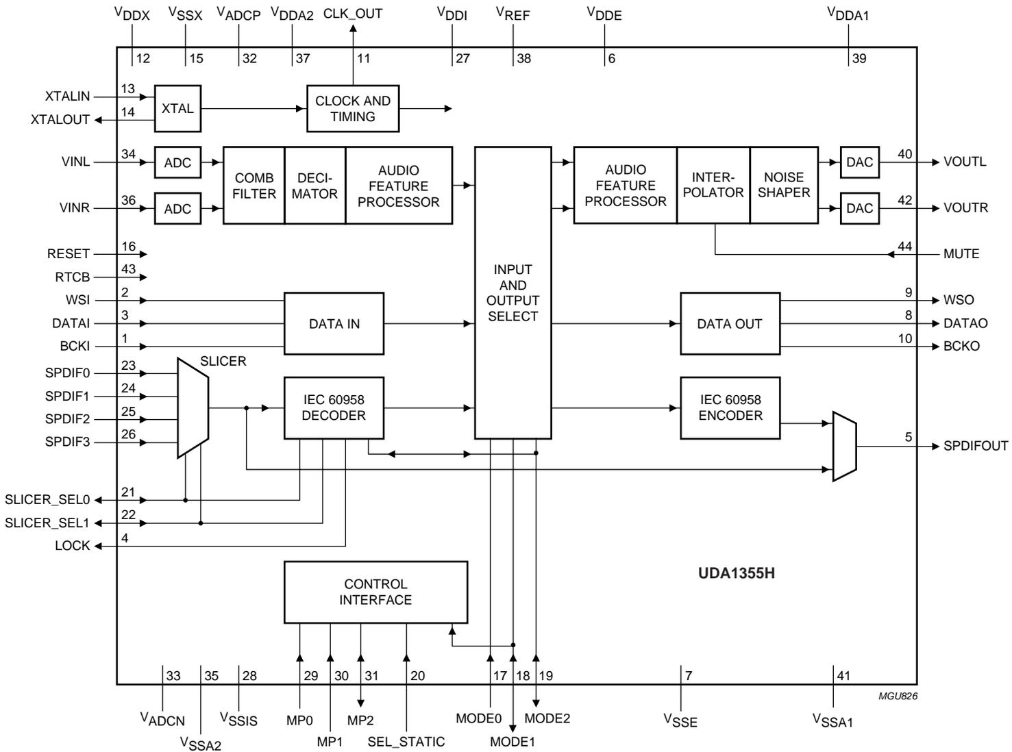
Fig.1 Block diagram.
