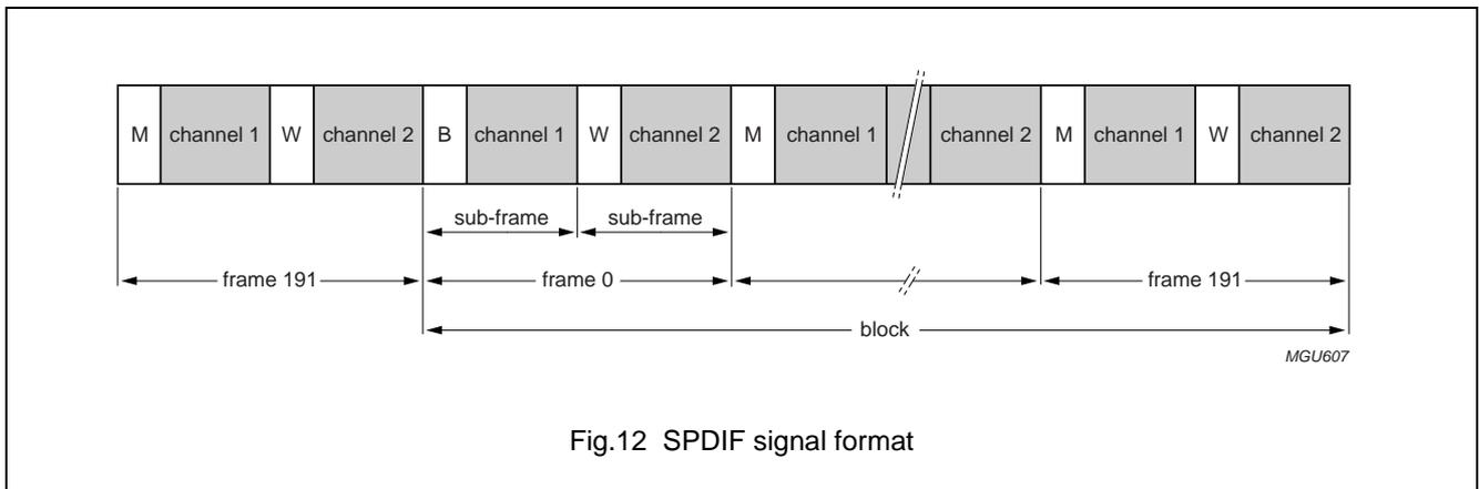
Fig.12 SPDIF signal format
