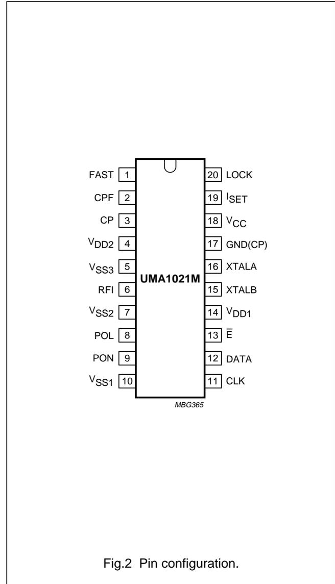
Fig.2 Pin configuration.
