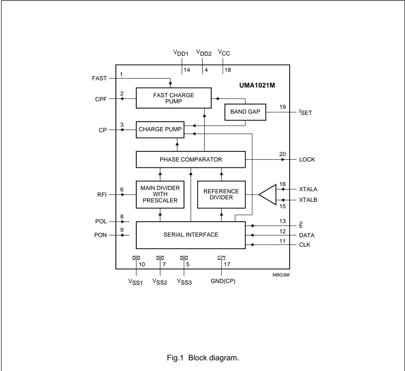
Fig.1 Block diagram.
