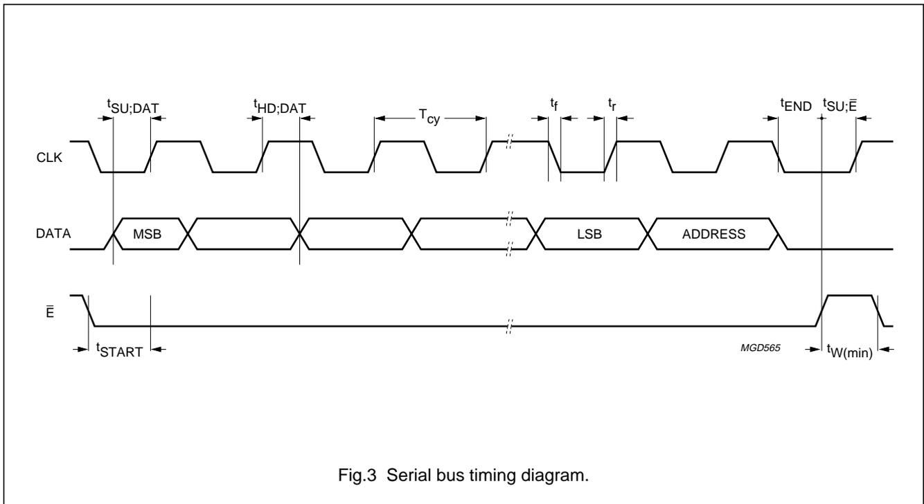
Fig.3 Serial bus timing diagram.
