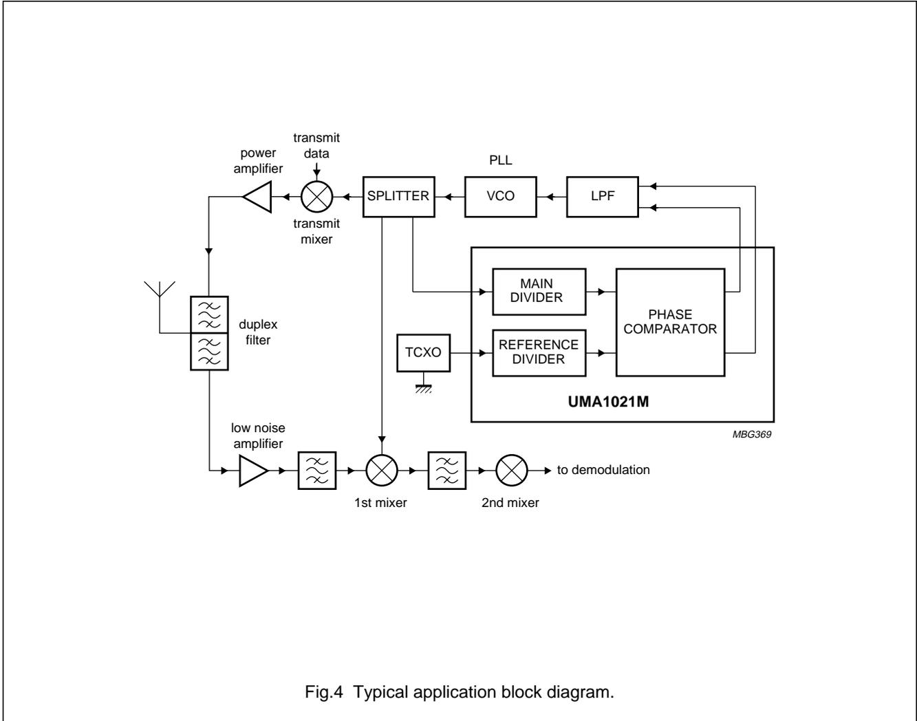
Fig.4 Typical application block diagram.
